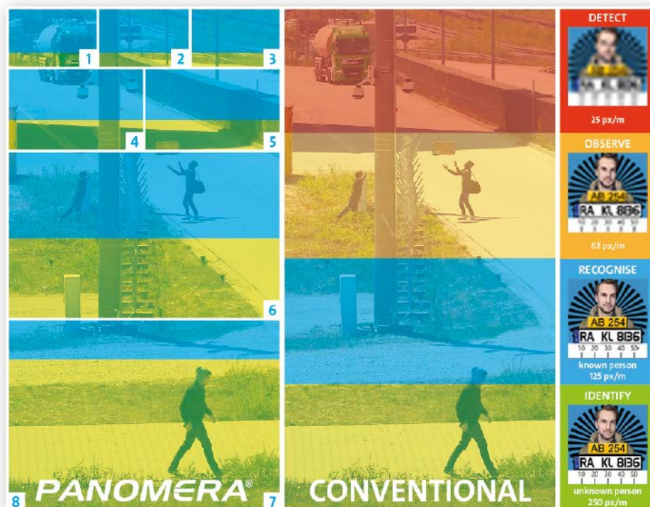
The values for the minimum resolution specified in DIN EN 62676-4 are the basis for any planning. With conventional technology, the laws of physics apply at full force. With Panomera, a much more even distribution of the resolution across the entire object space can be achieved
